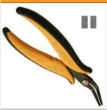
**PNB 2007:** Serrated flat long nose pliers bent at 45°. Thanks to its shape, it gives a wide angle of vision of the work area and suitable for the handling of components in difficult to reach areas. Steel thickness 3.0mm.
