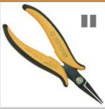
**PN 2007:** The PN 2007 is a serrated, flat long nose pliers ideal to be used in difficult to reach areas. Steel thickness 3.0mm.
